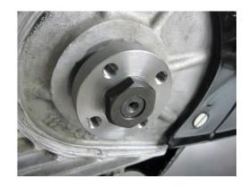
The position of the engine pulley should be as close as possible to the crankcase.
