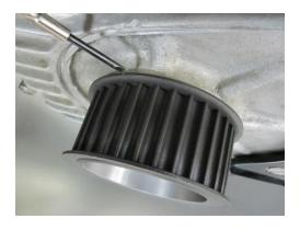
Lay belt over pulleys and slip engine pulley and the determined amount of shims over the adaptor.
