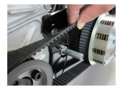
Temporarily attach all external parts that are necessary to get the clutch pulled. Leave the primary cover out.
