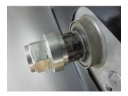
Install clutch assembly on maindrive gear.
