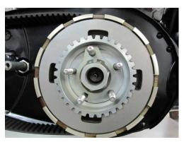
Install the pressure plate and insert spring retainers, springs and nuts.
