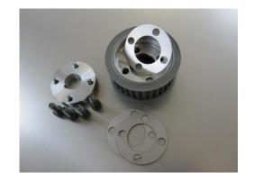
Slip the adaptor on the crankshaft and check if taper is fully seated. If key in crankshaft is too high, taper won't seat fully and you have to cut key to specification.
